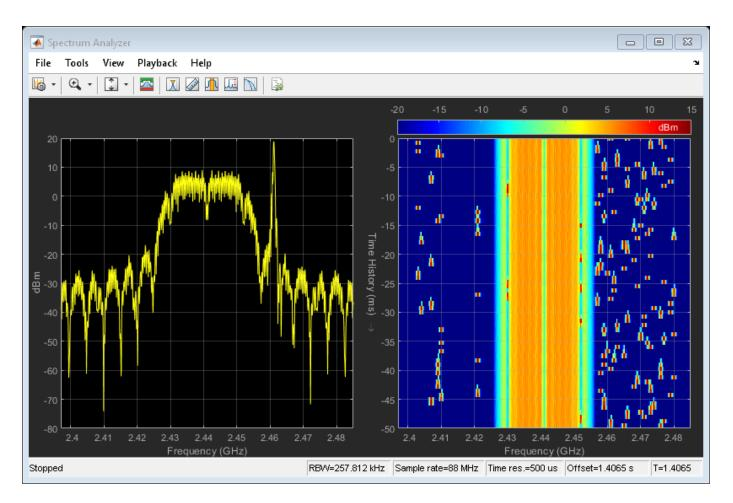
The preceding spectrum analyzer plot shows the spectrum of the Bluetooth waveform distorted with WLAN interference (in the frequency domain) and passed through the AWGN channel. The right-side plot shows the overlapping of Bluetooth packets with the interfering WLAN signal.
