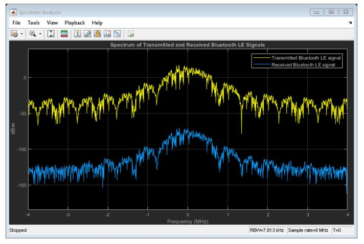
This example demonstrates an end-to-end Bluetooth LE simulation for different PHY transmission modes by considering the path loss model, RF impairments, and AWGN. The obtained simulation results display the path loss, estimated distance between the transmitter and receiver, and BER. The spectrum of the transmitted and received Bluetooth LE waveform is visualized by using a spectrum analyzer.
