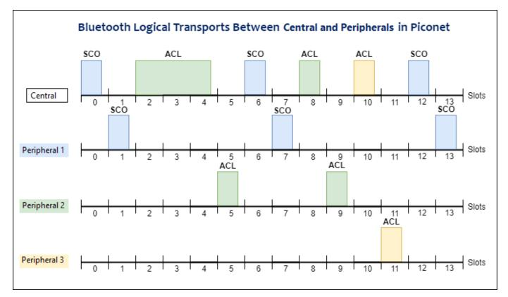
Bluetooth uses reserved time slots for communication between the nodes. The duration of each slot is 625 microseconds. The Central node initiates the transmission in even slots and extends the transmission to odd slots when transmitting a multislot packet. The Peripheral node initiates the transmission in odd slots and extends the transmission to even slots when transmitting a multislot packet.
