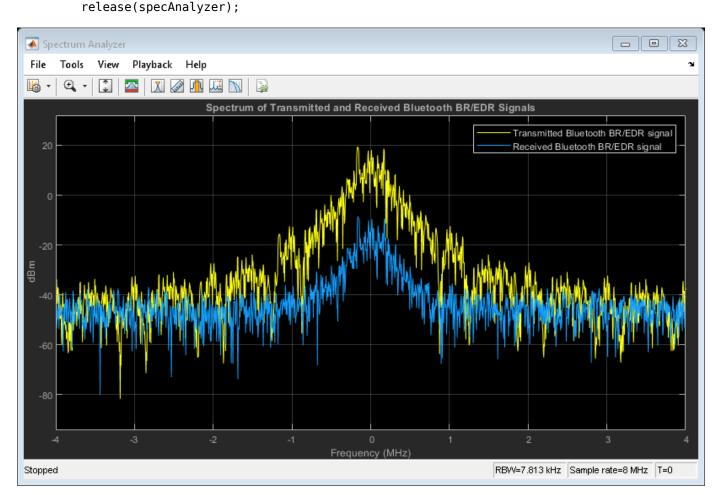
This example demonstrates an end-to-end Bluetooth BR/EDR simulation by considering the path loss model, distance between transmitter and receiver, RF impairments, and AWGN. The obtained
