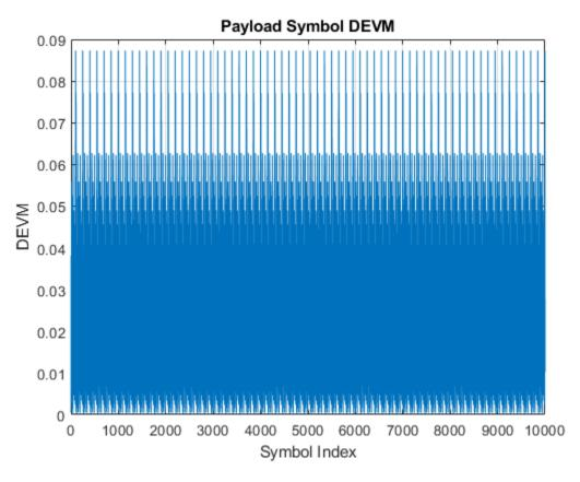
Expected peak DEVM for all pi/4-DQPSK symbols is less than or equal to 0.35 Result: Pass
