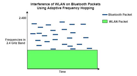
This procedure of remapping involves reducing the number of channels to be used by Bluetooth. The Bluetooth Core Specification [2] on page 5-0 require at least 20 channels for Bluetooth
