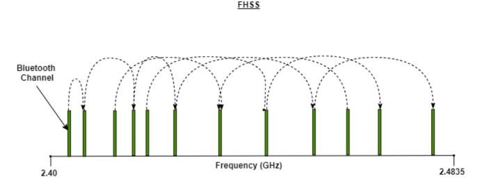
The transmitting and receiving Bluetooth devices adhere to a specific hopping sequence during a particular session so that the receiving device can anticipate the frequency of the next transmission. In this case, Bluetooth makes full use of the 2.4 GHz frequency spectrum.
