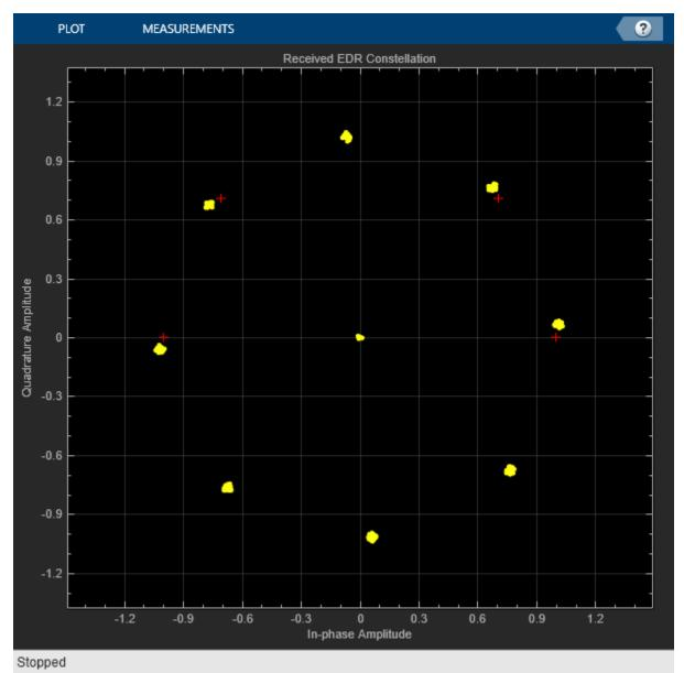
This example demonstrates the Bluetooth EDR transmitter test measurements specific to modulation accuracy and carrier frequency stability. The simulation results verify that these computed test measurement values are within the limits specified by the Bluetooth RF-PHY Test Specifications [1 on
