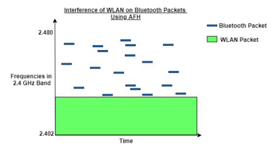
AFH dynamically alters the frequency hopping sequence to avoid the interference observed by the Bluetooth devices. AFH operates through these four processes.
