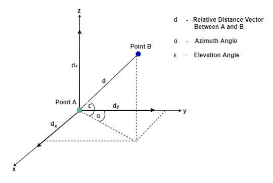
*d* is the relative distance vector between points A and B.  $d_x$ ,  $d_y$ , and  $d_z$  denote the components of *d* along *x*-, *y*-, and *z*-axis, respectively. Using this information, the azimuth angle ( $\alpha$ ) and elevation angle ( $\varepsilon$ ) between points A and B is calculated as:
