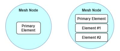
Elements consists of entities that define the functionality of a node and the condition of the element. Each element in a mesh node has a unique *unicast address* that enables each element to be addressed.
