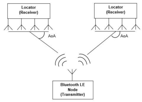
In the AoA method, the transmitter (Bluetooth LE node) transmits a direction finding signal using single antenna. The receiving device (locator), equipped with an antenna array, takes the IQ samples while switching between the antennas present in the array. The locator uses the IQ samples to calculate the AoA.
