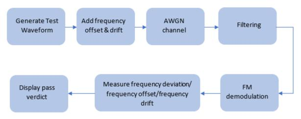
Generate Bluetooth LE test packets by using the bluetoothTestWaveform function. The test waveforms required for different test IDs are:
