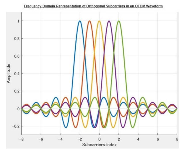
The use of narrow-band subchannels (compared to a single wideband channel) helps mitigate channel fading. As each subchannel operates at a low data rate, OFDM is very resilient to intersymbol interference and interframe interference. As data is transmitted simultaneously on multiple orthogonal subcarriers, OFDM can provide very high throughput. To further maximize the throughput, you can use OFDM with MIMO, extended rate physical (ERP), and multiuser (MU) technologies.
