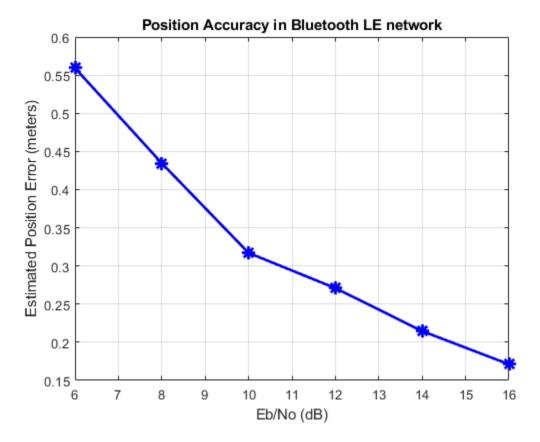
This example enables you to estimate the 2-D or 3-D position of a Bluetooth LE node by using the Bluetooth LE direction finding functionality. The example shows how to implement the triangulation method to calculate the angles between the locators and the Bluetooth LE node. The example also shows how to measure the positioning accuracy related to the Eb/No value by computing the distance between the estimated and actual node positions in an AWGN channel.
