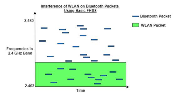
On the contrary, AFH enables Bluetooth to adapt to its environment by identifying fixed sources of WLAN interference and excluding them from the list of available channels. This figure shows the previous scenario with AFH enabled.
