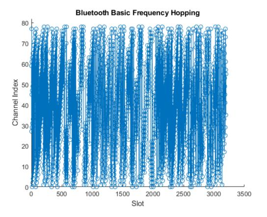
The preceding plot displays the selected channel index per transmission or reception slot using basic frequency hopping. In this case all of the channels are used channels.
