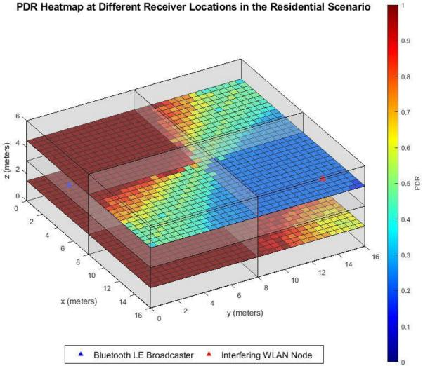
You can analyze the improvement in PDR in the presence of interference by changing the configuration parameters. To observe an increase in PDR, you can:
