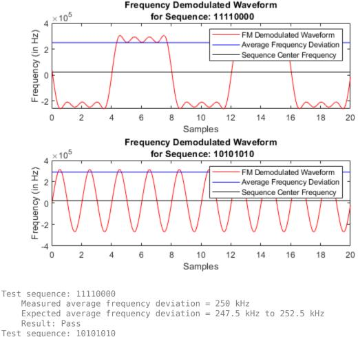
Expected 99.9% of all maximum frequency deviation > 185000 kHz Result: Pass Ratio of frequency deviations between two test sequences = 1.163 Expected Ratio > 0.8 Result: Pass
