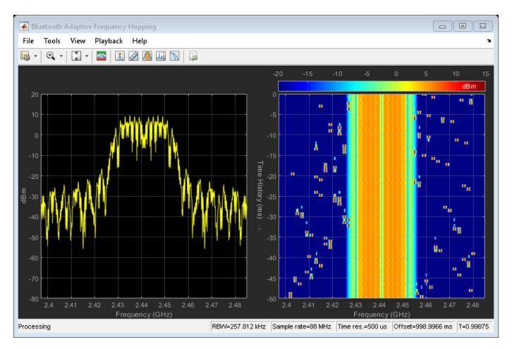
In the previous plot, you can observe that the transmission of Bluetooth packets does not overlap with the WLAN signal. AFH excludes the channels that are sources of WLAN interference and reassigns the transmission of Bluetooth packets on channels with relatively less interference.
