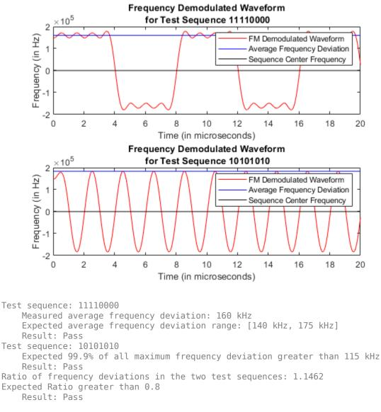
This example demonstrates the Bluetooth BR transmitter test measurements specific to modulation characteristics, carrier frequency offset, and drift. The simulation results verify that the computed test measurement values are within the limits specified by Bluetooth RF-PHY Test Specifications [1 on page 4-0 ].
