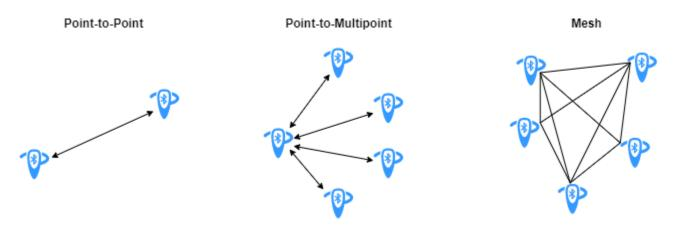
Devices using one-to-one communication operate in a Bluetooth *piconet*. As shown in this figure, each piconet consists of a device in the role of *Central*, with other devices in the *Peripheral* or *Advertiser* roles. Before joining the piconet, each *Peripheral* node is in an advertiser role. Multiple piconets connect to each other, forming a Bluetooth *scatternet*.
