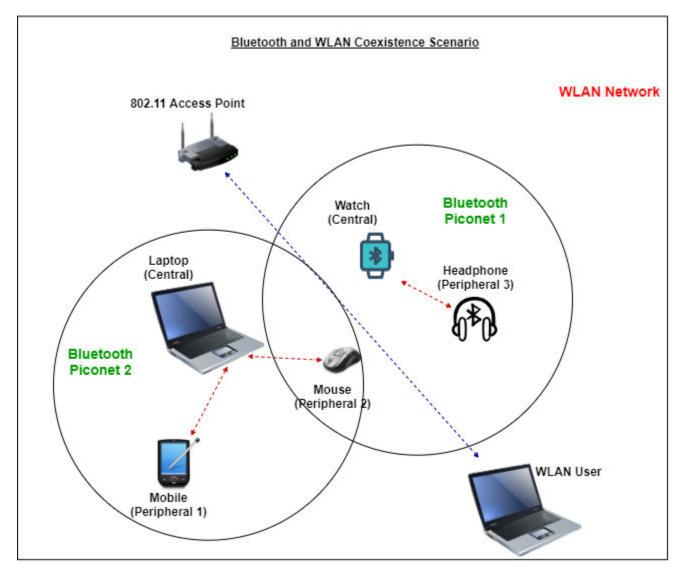
If the transmission in piconet 1 is overlapped in time and frequency by transmissions from piconet 2 and/or the WLAN, a Bluetooth packet can be lost. This figure shows how the Bluetooth and WLAN devices share the 2.4 GHz frequency spectrum.
