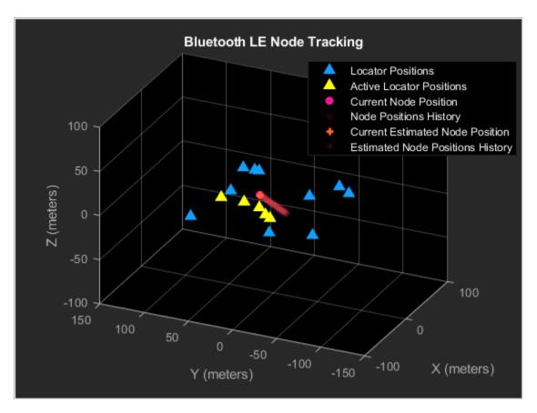
This example enables you to estimate the 2-D or 3-D position of a Bluetooth LE node using the direction-finding functionality and location estimation techniques. The example also measures positioning accuracy at each node position.
