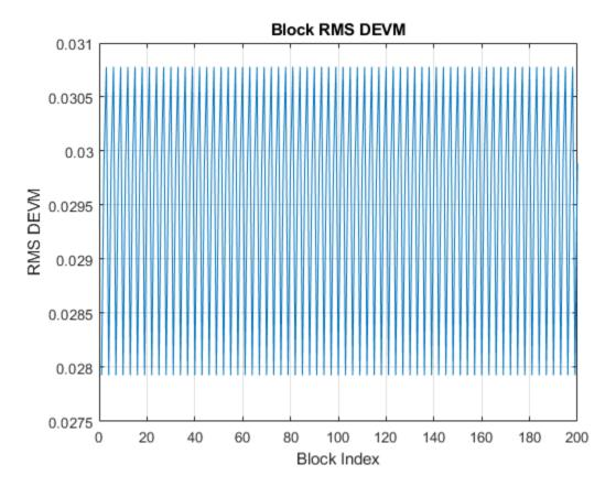
Expected RMS DEVM for all pi/4-DQPSK blocks is less than or equal to 0.2 Result: Pass
