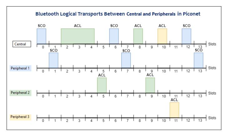
The Central polls a Peripheral with a poll packet (if no data exists) or a data packet in a Tx slot, and the Peripheral responds to the polling. The Central can poll any Peripheral of the SCO or ACL logical transport. For SCO links, the Central reserves the slots for the dedicated SCO Peripheral. The Central polls the ACL Peripherals in the remaining slots. The Peripheral responds to the Central with a data packet or a null packet.
