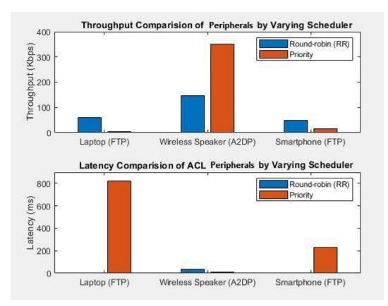
For the RR scheduler, the throughput and latency values are approximately same for the laptop, wireless speaker, and smartphone. The QoS-based priority scheduler achieves the desired throughput and low latency of the wireless speaker (Peripheral 2).
