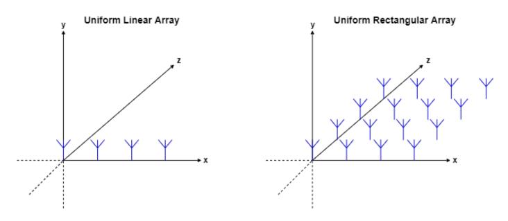
Calculating the elevation and azimuth angles of the signal relative to a reference plane is common in these antenna arrays. This figure shows the concept of azimuth and elevation angles.
