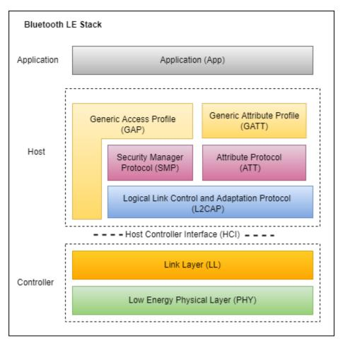
The L2CAP layer in Bluetooth LE corresponds to the higher sub-layer i.e. Logical Link Control (LLC) of the Data Link Layer in the OSI reference model. The L2CAP is above the PHY and Link Layer of Bluetooth LE. The Bluetooth LE specification optimized and simplified the L2CAP when compared to classic Bluetooth.
