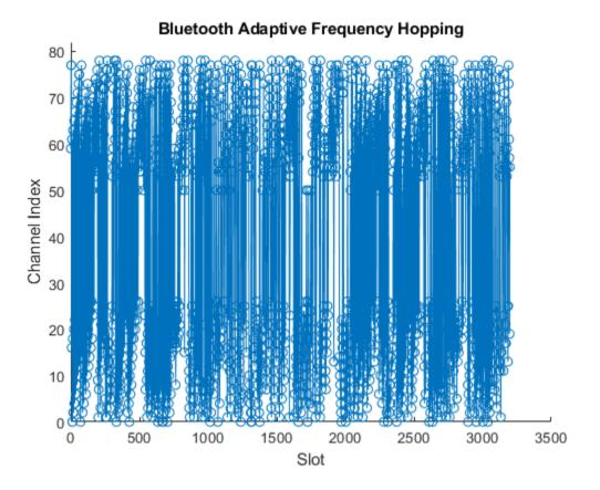
The preceding plot displays the selected channel index per transmission or reception slot using AFH. To minimize the packet and bit errors in the wireless channel, AFH selects only used channels for transmission or reception of Bluetooth BR/EDR waveforms
