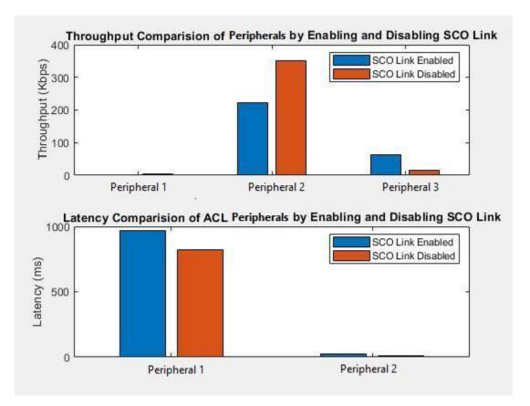
The presence of the SCO link degrades the throughput and latency performance of ACL Peripherals. And also, the wireless speaker (Peripheral 2) cannot achieve the required throughput if an SCO Peripheral in the piconet exists, even if you use a QoS-based priority scheduler. Because acknowledgement for SCO packets is not required, the latency is calculated only for the ACL Peripherals.
