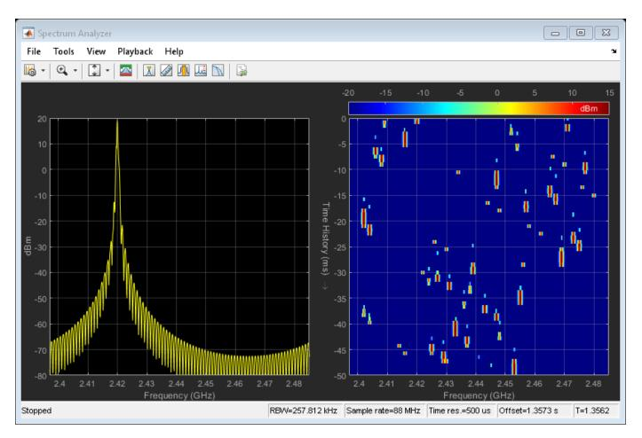
The preceding Spectrum Analyzer plot shows the spectrum of the Bluetooth waveform distorted with WLAN signal interference (in the frequency domain) and passed through the AWGN channel. The right-side plot shows the overlapping of Bluetooth packets with the interfering WLAN signal. The WLAN waveform in the plot is present throughout the simulation.
