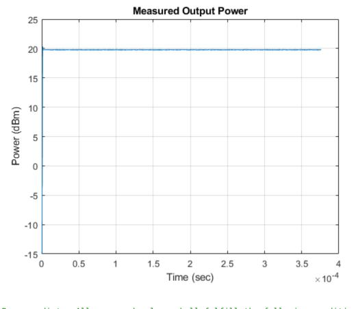
% Pass verdict - All measured values shall fulfill the following conditions: % % \* Peak power <= (Average power + 3 dB) % \* -20dBm <= Average power <= 20dBm %
