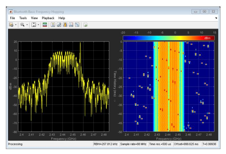
In the previous figure, the plot on the left shows the spectrum of the Bluetooth BR/EDR waveform distorted with WLAN interference in the frequency domain and passed through the AWGN channel. The plot on the right shows that the WLAN signal is present from -10 to 10 MHz. The results show that Bluetooth packets with the interfering WLAN signal overlap.
