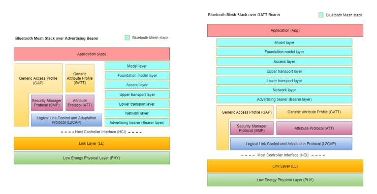
The Bluetooth mesh stack consists of these layers:
